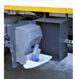
Hand Wash facility
